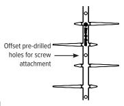
*Tie Down:* For pipes and other areas, secure bird spike strips with nylon ties by wrapping and securing the tie around the base of the bird spike strip.
