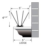
For wide areas, multiple rows of bird spike strips may need to be installed. Install bird spike strips with 1" overlap.
