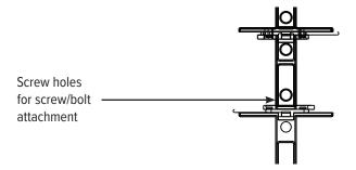
**For Wood:** Use wood screws to secure bird spike strips to wood surfaces. Following pre-drilled holes along the strip base, screw into the end of each bird spike strip tightly; place one wood screw at least every six inches along the strip base.
