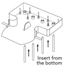
Insert rods through the bottom of the tray until they "snap" into place.
